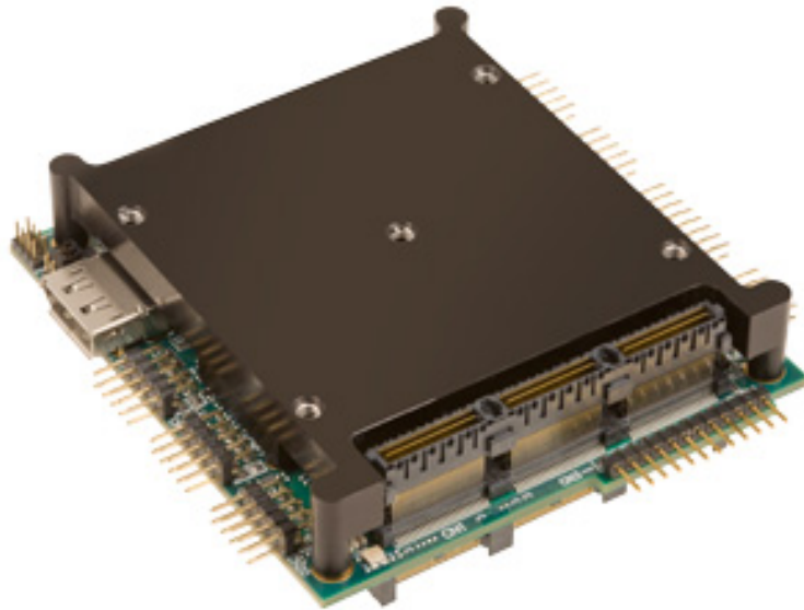
Figure 27: The CPU with the heat sink to be linked to the wall of minieuso
